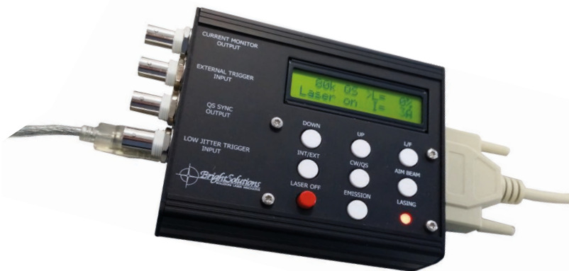
Digital control box for simplified remote control
