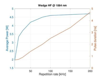
In principle, the calculation is quite simple, even though some considerations should be done, based on the actual temporal profile of the laser pulse. By assuming a train of continuously repeated periodical square pulses with repetition rate fr, pulse duration to and average power PAV, the pulse energy EP and peak power PP calculation is trivial, with pulse energy given by the ratio between average power and repetition rate and peak power given by the ratio between energy and pulse duration:
