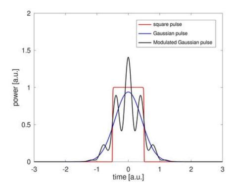
By considering for example the performance curves of a standard Bright Solutions's Wedge HF laser at 1064 nm, the average power at 100 kHz is 4.6 W and pulse duration is about 2.5 ns, giving a peak power of ~ 18 kW.
