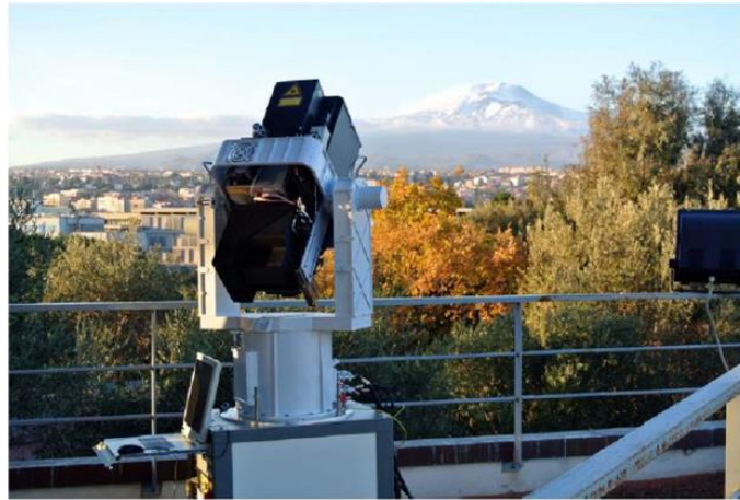
Actively Q-Switched DPSS laser is monitoring Etna volcano from a remote station in Catania, Sicily
