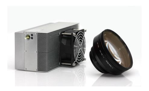
In order to obtain grayscale images with <u>Sol</u> laser, a fast output power modulation is needed. This fast Pulse Energy Modulation can be achieved connecting a dedicated input signal present in the IO electronic interface of the laser to an analog output port of the marking hardware that can be modulated from 0 to 5V according to software commands.
