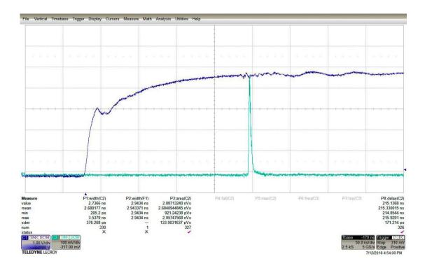
The oscilloscope screenshot above shows an example of jitter measurement for a Bright Solutions 2.7ns-long low-jitter airborne LiDAR illuminator. The blue curve is the trigger IN signal, while the green one is the laser pulse detected by a fast photodiode. The standard deviation of the delay of the laser pulse respect to the rising edge of the trigger IN signal is the jitter.
